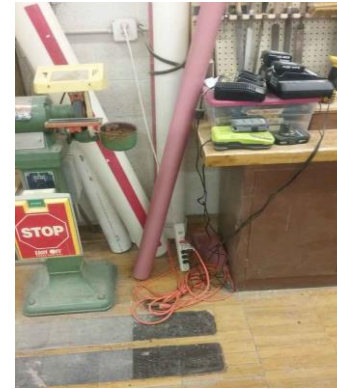
Extension cord being used as permanent wiring.
